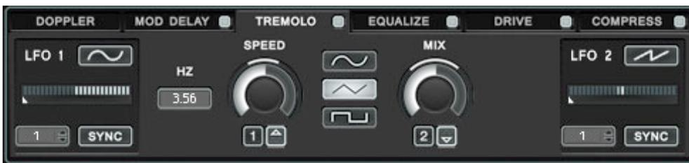
Tremolo offers control over speed and mix. Both controls can be modulated via the two LFO's in the same way as the mod delay. It is also possible to choose between three different tremolo shapes.
