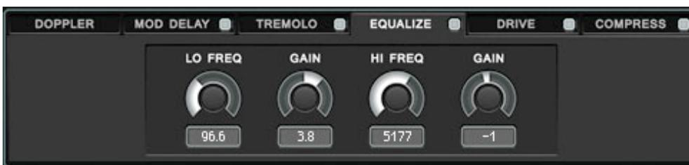
Equalize is a basic high and low shelf equalizer. You can select a specific low or high frequency value and increase or decrease it's gain.
