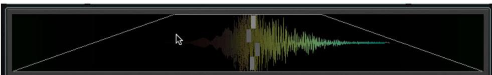
In the scope display it is possible to control the master fade. The master fade is an overall volume fade imposed on the whole doppler event. This ensures a smooth start and end modulation. The master fade becomes especially useful when the source mixer is operating in random mode, where the audio can be unpredictable.
