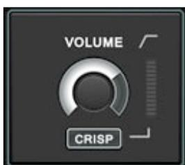
Controls the master output volume of the instrument. At the end of it's signal chain is a brick wall limiter indicated through the gain reduction meter. The limiter can operate in three different modes: Slow, Firm and Crisp. Crisp has an ultra short attack time and may lead to some additional digital distortion. This can be desired to get some extra crunchiness.
