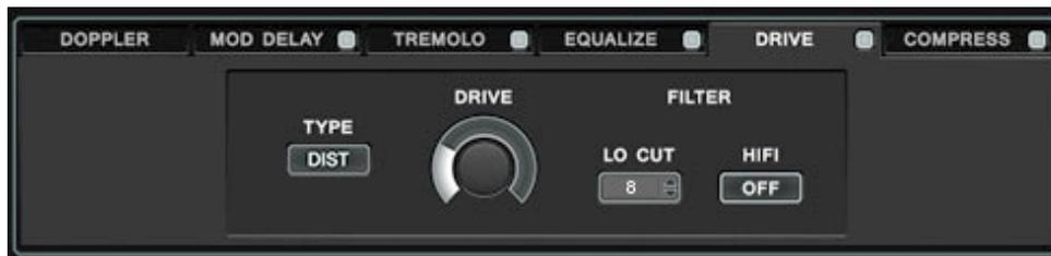
You can select between drive and saturation mode. The big encoder allows you to dial in the drive effect. There is also some additional filtering offered. The additional drive effect may lead to an increased volume of the lower frequencies. The low cut filter could help balancing here. There is also a HiFi filter offered which lowers the mid range frequencies.
