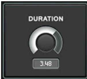
The master duration defines the length of the whoosh sound effect. When changing the duration all the synchronized parameters follow. (Effect LFO's and granular playback position).
