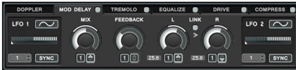
Mod Delay offers control over mix, feedback, left and right channel delay time. All the four parameters can be modulated by selecting one of the two LFO's. Which LFO can be selected in the number fields under the encoders. Add the desired modulation amount through click and drag in the little arrow spinner knobs. Special about the mod delay is that the delay time only goes up to 80 ms which is perfect for creating flanging, chorus and metallic delay effects.
