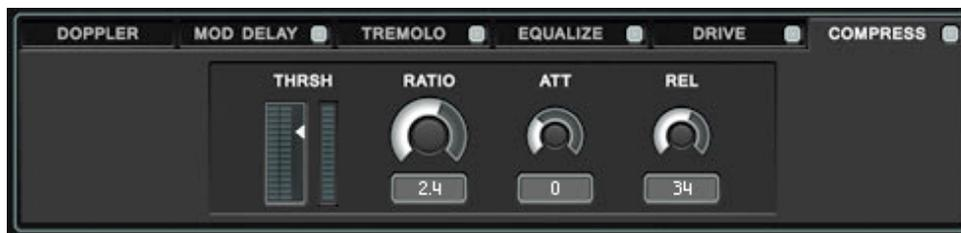
Compress is a basic compressor and offers control for compression, threshold, ratio, attack and release time.
